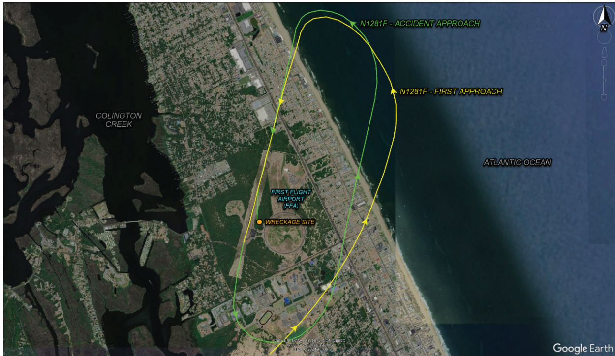
Figure 1- Preliminary ADS-B data showing the airplane's flight track during the accident approach (green line) and the previous approach to runway 21 (yellow line).
